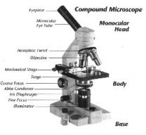
Base: the horizontal, oval-shaped part upon which the microscope rests.
