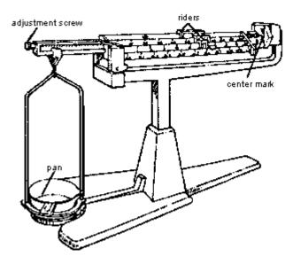
which is marked off in the smallest increments, is not notched. Slide the rider on this beam until the pointer swings an equal distance on each side of the zero on the scale.
